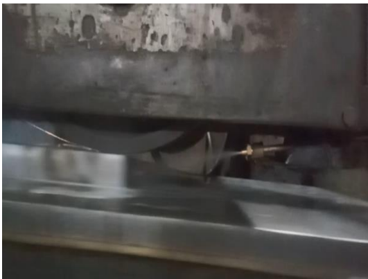
Fig. 2 Mist spray in MQL grinding process
